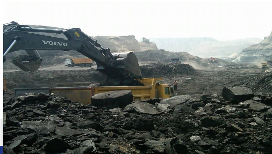
Removal of OB for Rajmahal Area
