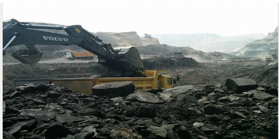
Removal of OB for Rajmahal Area
